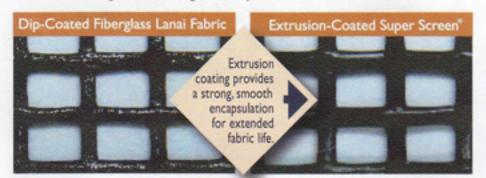
The polymer and polyester properties of Super Screen' defy deterioration. In a similated seven-year weathering test, Super Screen' lost only 1% of its original strength. It remained 3 times stronger than fiberglass screen.
